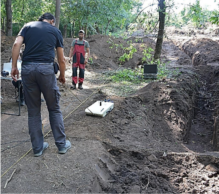
Photo no. 10 – utilizing a magnetometer to demarcate the surface of a mass grave already identified in an exploratory ditch. Photo used with the permission of the Military Prosecutor's Office in Iași.
